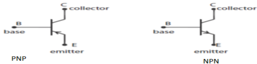
Figure 6.23: Symbols for PNP and NPN transistors.
